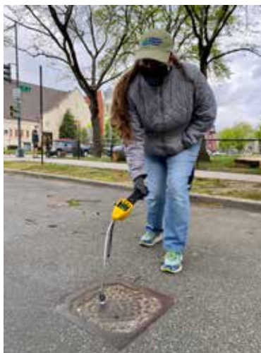
ANS staff checking for methane gas leaks near an elementary school in Washington, DC. Learn more about the Beyond Gas campaign to move away from climate-harming methane in upcoming workshops.
