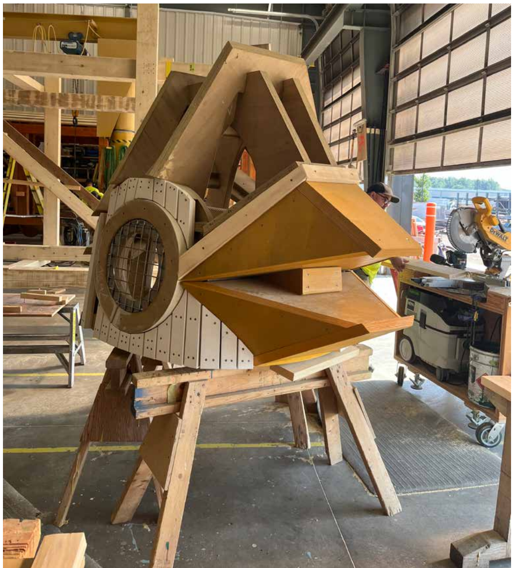
Our Wood Thrush accessible climbing feature taking shape in the workshop of fabricator Earthscape Play.
